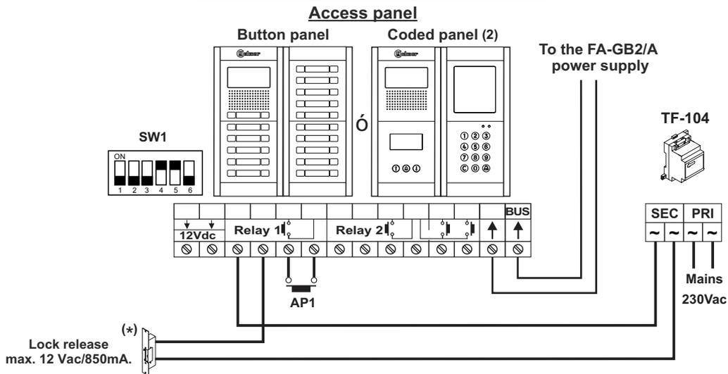
(\*) Important: Place the varistor supplied with the sound module directly onto the terminals of the lock release.
