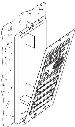
The frame can now be tilted horizontally to enable sound module and button module connection and setting.
