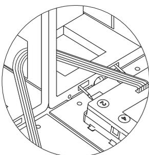
Between EL610D button modules in different embedding boxes, insert one end of the short connection cable into the lower connector of the final EL610D module in the first embedding box and the other end into the middle connector of the last EL610D button module situated at the bottom of the second embedding box, as shown in the drawing.
