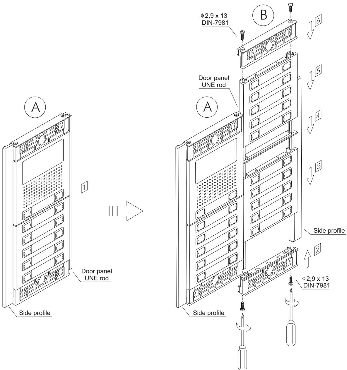
**IMPORTANT:** Once the adjustments are completed, stick the adhesive joint (enclosed with the N60XX CMPL end piece set) to the door panel UNE rod.
