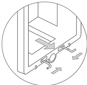
Insert the spring hinge which attaches to the product in the embedding box, as shown in the drawing.
