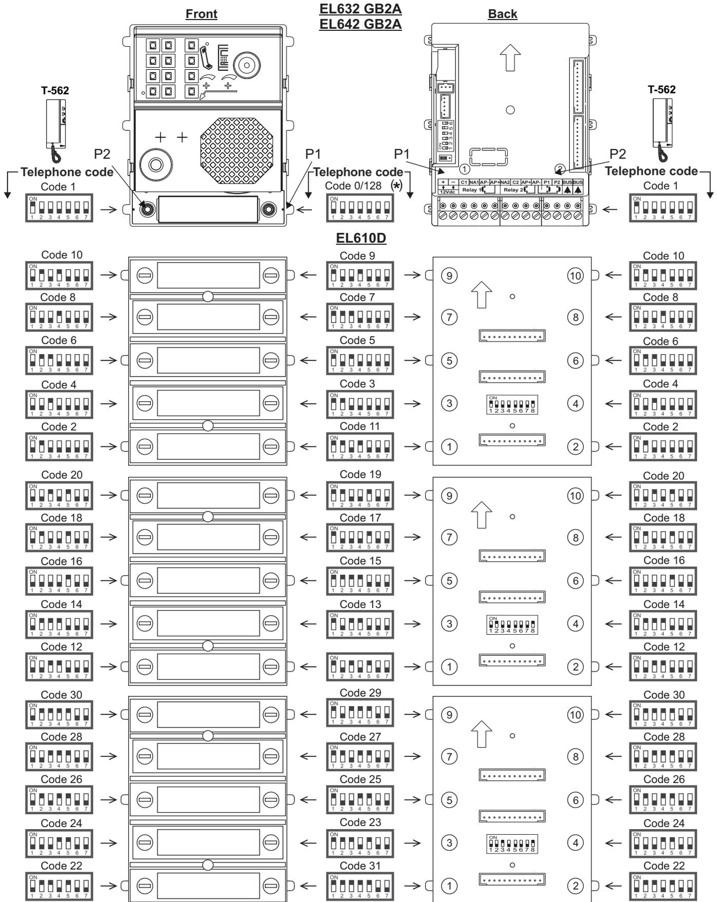
(\*) -In door panel systems with call pushbuttons, the first address on the telephone is 'Code 0'.
