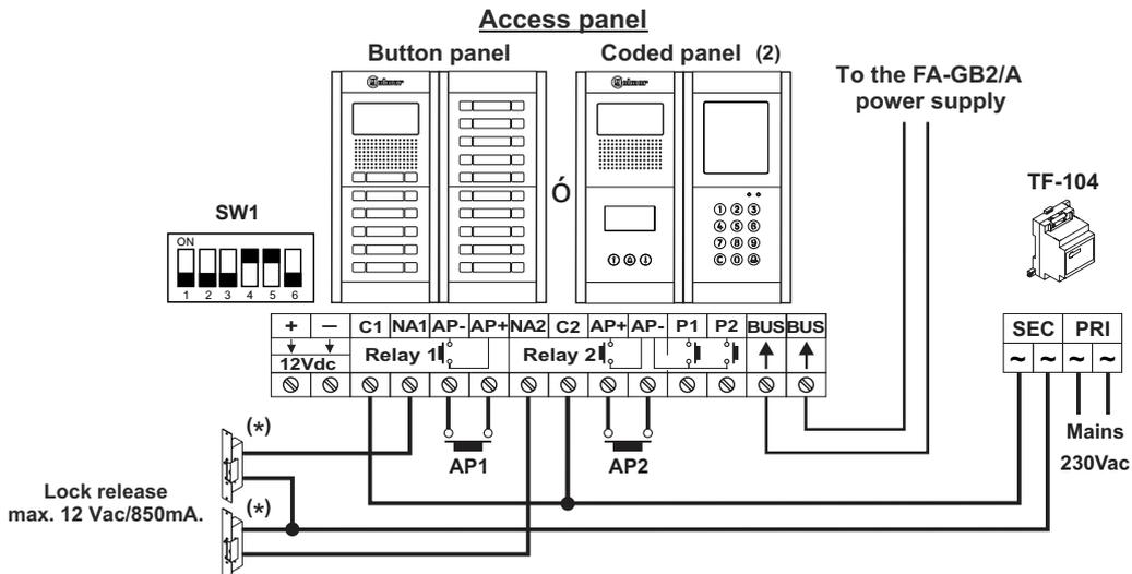
(\*) Important: Place the varistors supplied with the sound module directly onto the terminals of the lock release.
