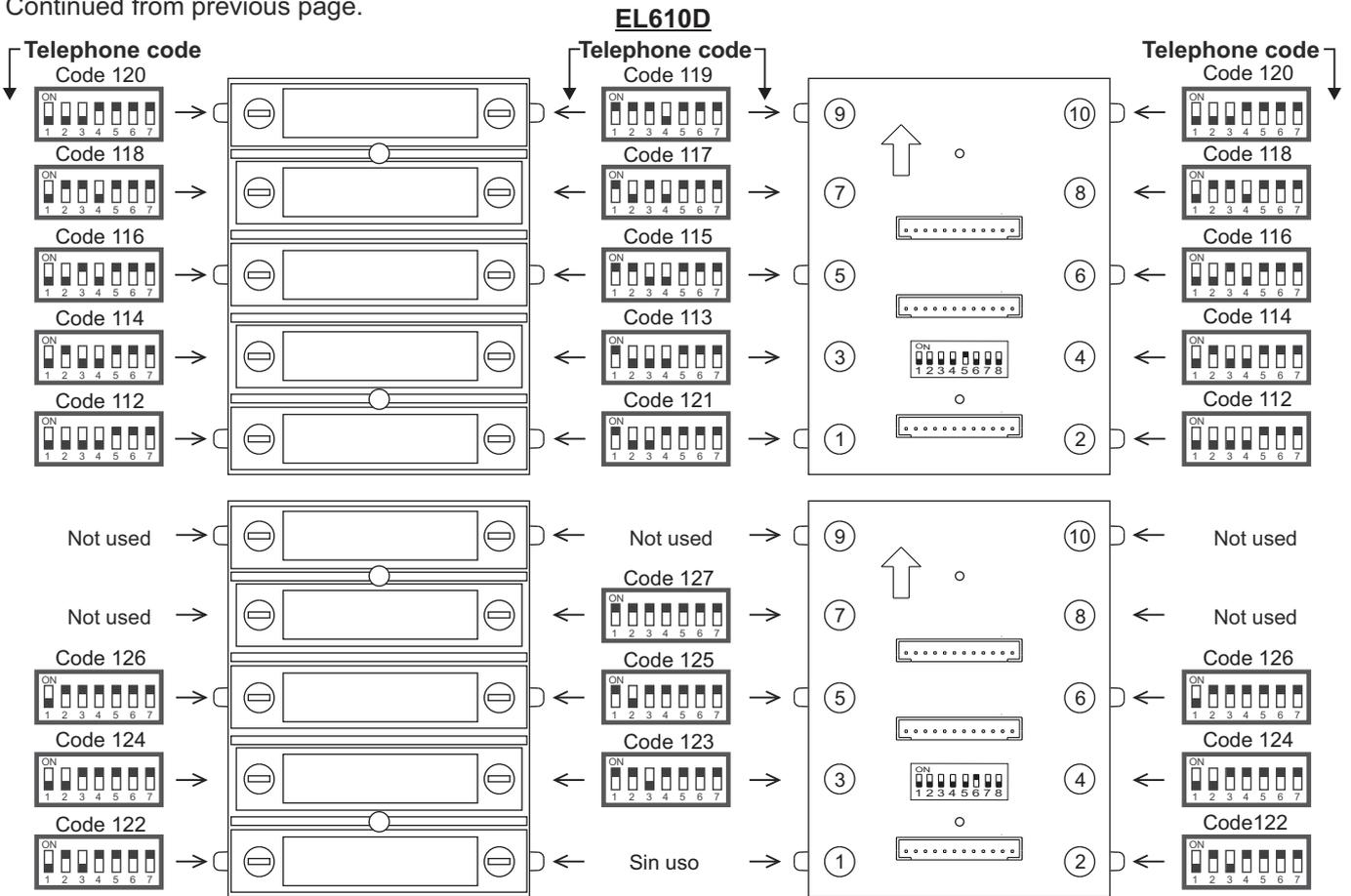
**IMPORTANT:** The T562/TNHEA telephone's DIP 10 should be set to ON.
