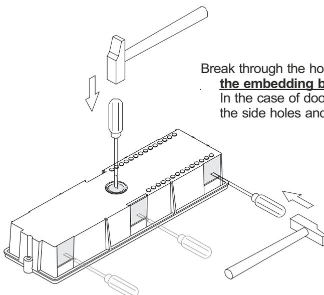
Break through the hole to allow **entry of cables through the bottom part of the embedding box.**
