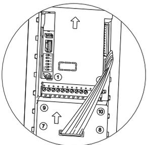
Insert one end of the short connection cable supplied with the EL610D product into the sound module connector and the other end into the connector situated at the top of the EL610D button module, as shown in the drawing.
