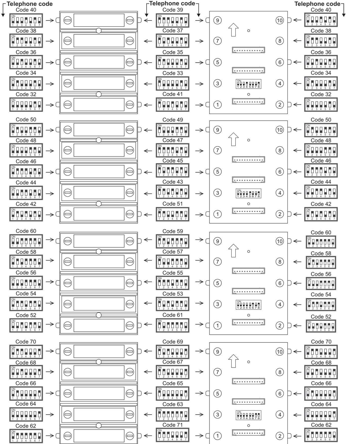
**IMPORTANT:** The T562/TNHEA telephone's DIP 10 should be set to ON.
