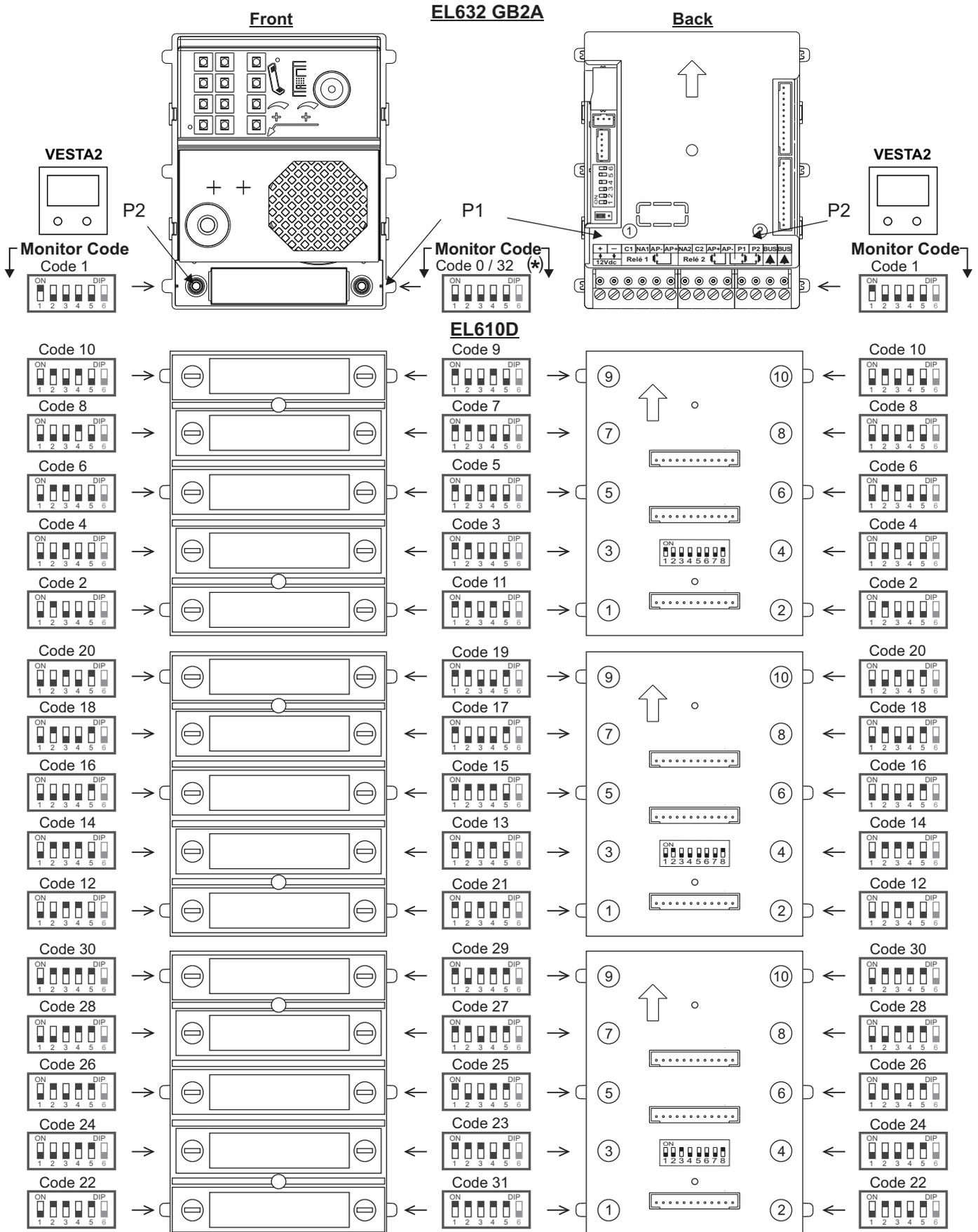
(\*) -In door panel systems with call pushbuttons, the first address on the monitor is 'Code 0'.
