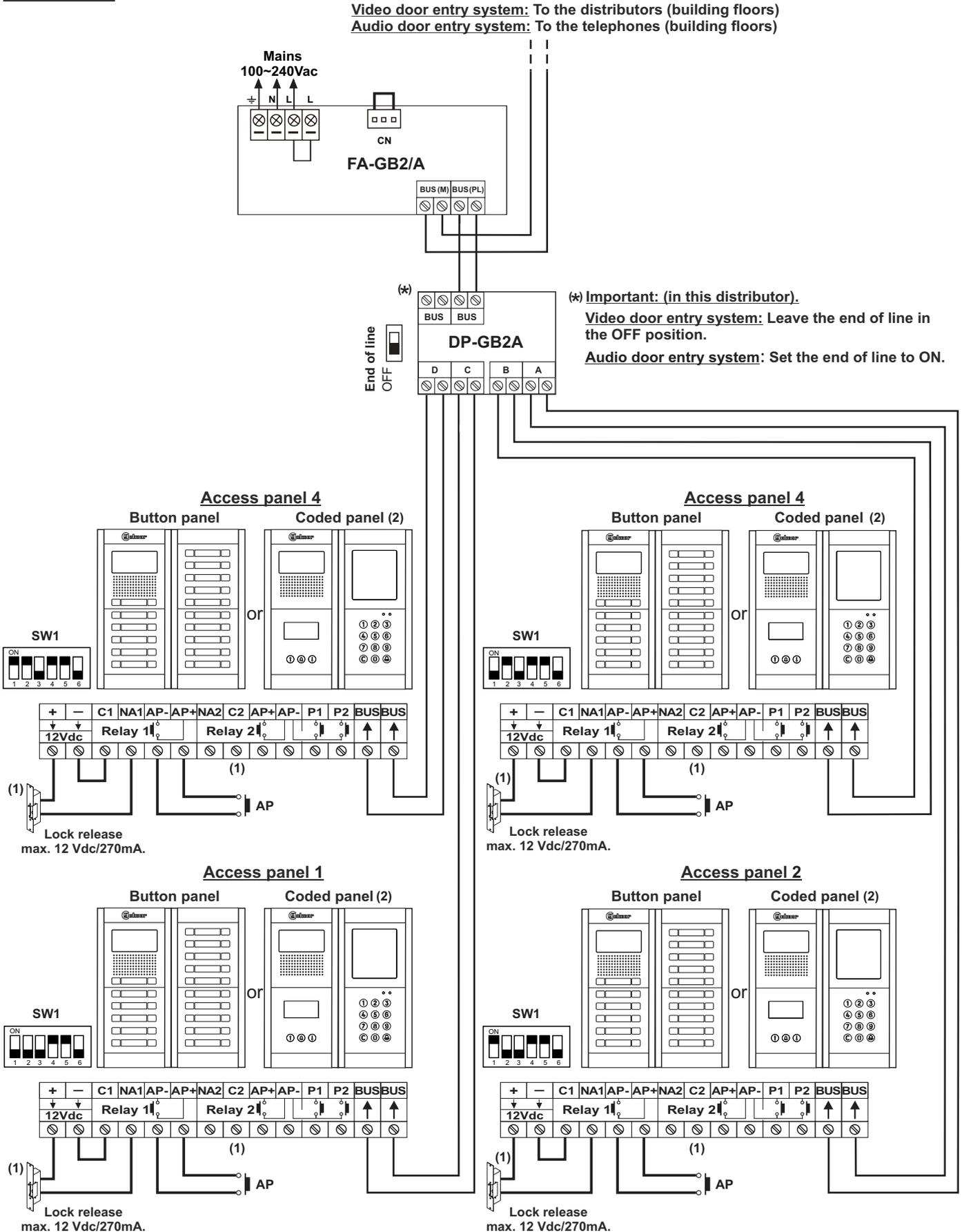
(1) **Important:** For the connection of an AC lock release or a 2nd lock release, see page 43.
