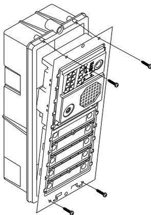
Once the wiring and configuration work is done, fix the frame to the embedding box using the screws supplied.
