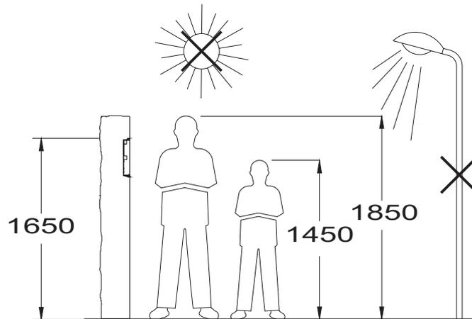
Make a hole in the wall to position the top of the door panel at a height of 1.65m.
