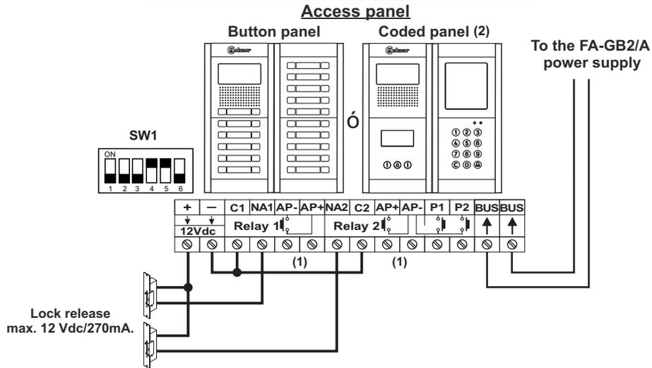
(1) Important: With 2 d.c. lock releases, it is not possible to use the "AP" door release buttons.
