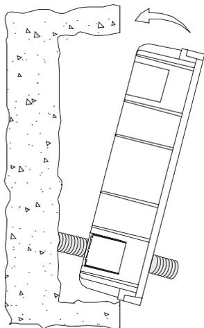
Pass the cable through the hole made in the embedding box. Embed the box and ensure that it is level and flush. Once the embedding box is positioned, remove the protective stickers from the door panel's fixing holes.
